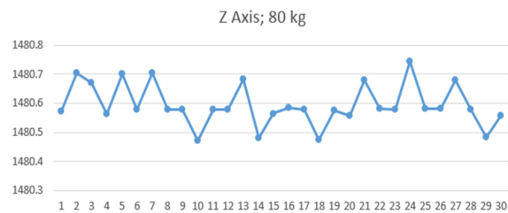
Fig. 25. Effect of linearization on robot position on the z axis for 80 kg payload in the end-effector
