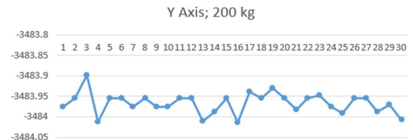
Fig. 34. Effect of linearization on robot position on the y axis for 200 kg payload in the end-effector
