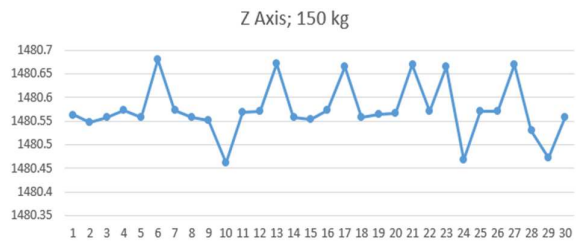
Fig. 29. Effect of linearization on robot position on the z axis for 150 kg payload in the end-effector
