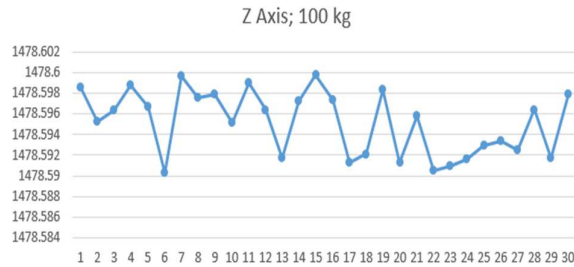
Fig. 10. Deviations of the target position on the z axis with 100 kg load in the end-effector
