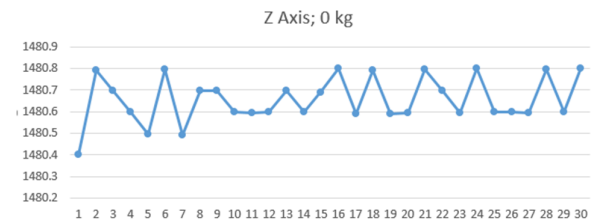
Fig. 4. Deviations of the target position on the z axis with 0 kg load in the end-effector
