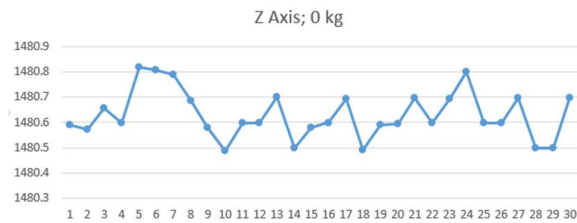
Fig. 21. Effect of linearization on robot position on the z axis for 0 kg payload in the end-effector
