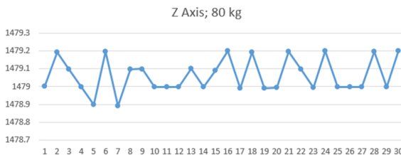
Fig. 8. Deviations of the target position on the z axis with 80 kg load in the end-effector
