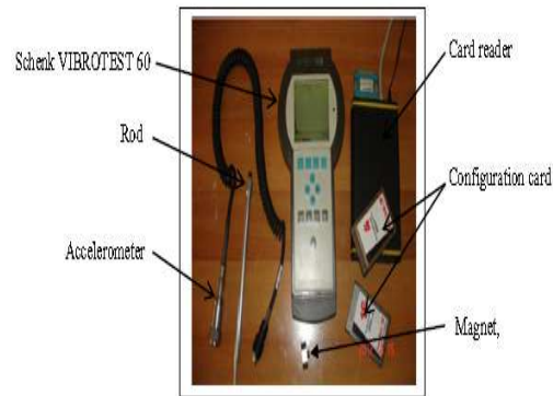
Fig. 3. The components of VIBROTEST 60 with vibration sensors [22].
