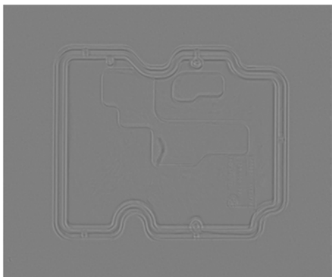
Fig. 9. Lack of image sharpness due to unstable acquisition conditions (overexposure, vibrations, etc.)
