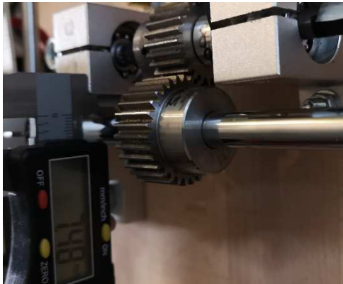
Fig. 14. Measuring distance between shafts
