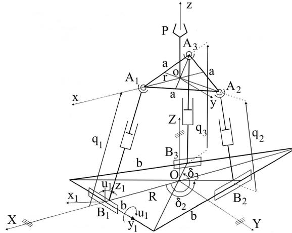
Fig. 1. Kinematic scheme of the 3RTPS parallel manipulator
