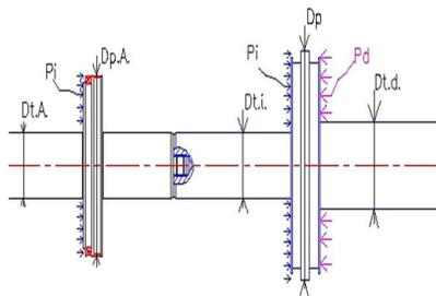
Figure 8 – The structure of the pistons which dual acts
