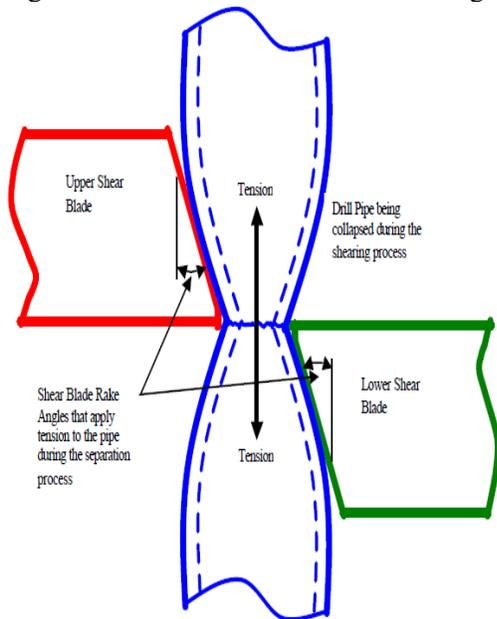
Figure 1 – Upper and lower cutting knives that crush the drill pipe and start cutting (or breaking)
