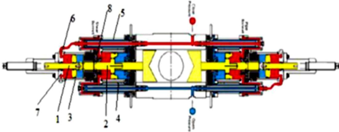
Figure 7 – The representation of the booster which shows hydraulic fluid line red for closing
