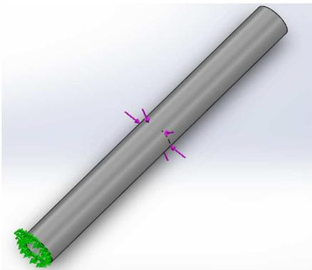
Figure 3 – Drill pipe sample 5in G-105 geometric model
