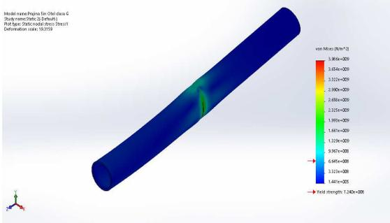
Figure 5 – Stress map for 5in G-105 drill pipe
