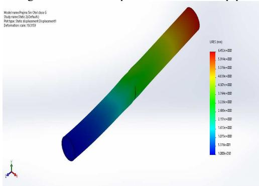
Figure 6 – Displacements map for 5in G-105 drill pip
