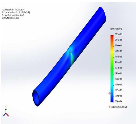
Figure 9 - Stress map for 5in S-135 drill pipe
