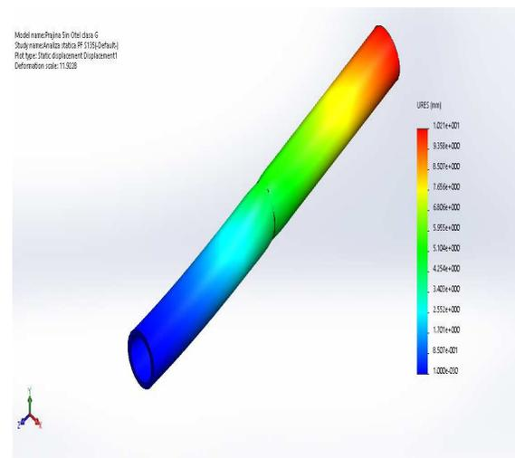
Figure 10 – Displacements map for 5in S-135 drill pipe
