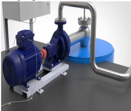
Fig. 9 The pump, electric motor, and the sensor
