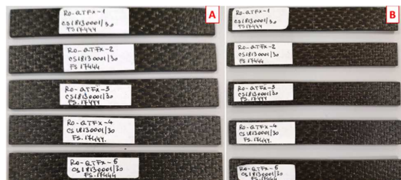
Fig. 7. Specimens in the 0° plane before and after flexural testing
