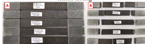
Fig. 4. Specimens in the 90° plane before and after tensile testing
