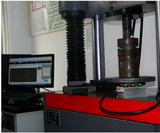
Fig. 23 Static metal testing machine for traction and compression type WEW - 600D
