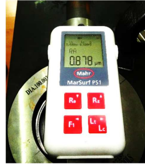
Fig. 19. Recording the initial roughness of the cylinder before pressing
