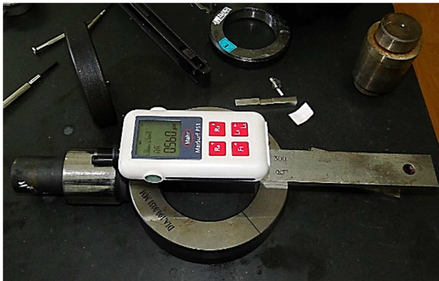
Fig. 20. Cylinder roughness recording after assembly ( R_a = 0.560 \mu\text{m} )
