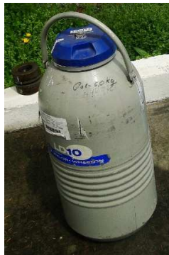
Fig. 16. Dewar vessel for storing liquid Nitrogen ( N_2 )
