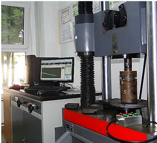
Fig. 15. Machine for static testing of metals at traction and compression
