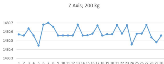
Fig. 33. Effect of linearization on robot position on the z axis for 200 kg payload in the end-effector
