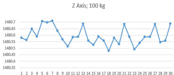
Fig. 27. Effect of linearization on robot position on the z axis for 100 kg payload in the end-effector
