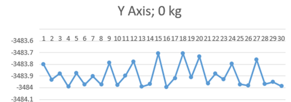
Fig. 5. Deviations of the target position on the y axis with 0 kg load in the end-effector
