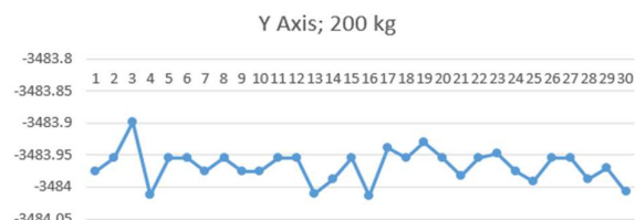
Fig. 34. Effect of linearization on robot position on the y axis for 200 kg payload in the end-effector
