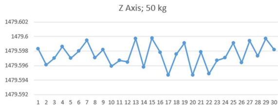
Fig. 6. Deviations of the target position on the z axis with 50 kg load in the end-effector
