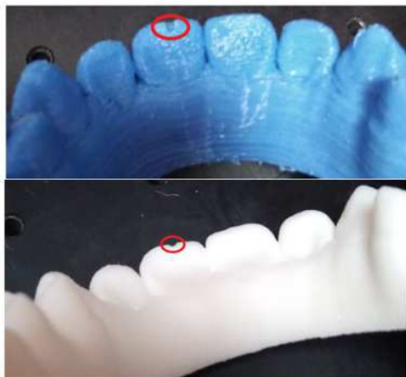
Fig. 4. Effect of testing on FDM dental model (top) and SLS dental model (bottom)
