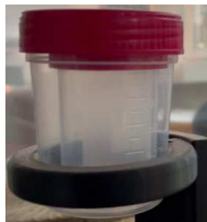
Fig. 5. SC isolator cap screwed in the “correct” position
