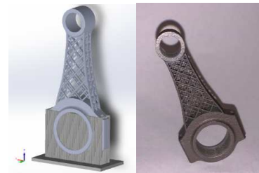
Fig.14. Theoretical vertical build orientation and use of supports. Connecting rod manufactured using SLM technology
