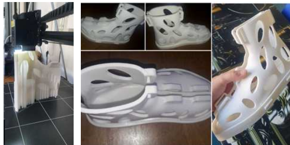
Fig.11. Realized part before and after support removal
