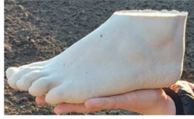
Fig. 1. The mold required for designing of foot orthosis
