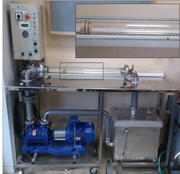
**Fig. 2.** Laboratory stand with cavitation chamber shown in enlargement [16].
