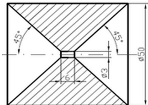
Fig. 4. Converging-diverging nozzle used in the experiment [16].
