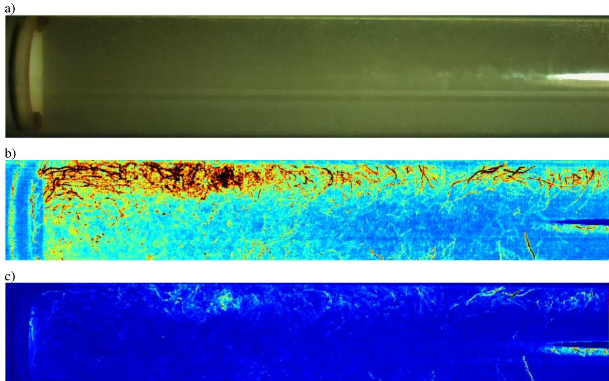
**Fig. 6.** Exemplary photograph of cavitating flow captured with a high-speed camera (with lasers turned off), as well as two variability maps (b and c) obtained based on image processing of the whole series of those images [9].
