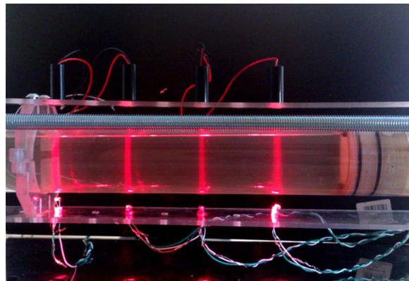
**Fig. 3.** The cavitation chamber with mounted lasers and photoresistors.
