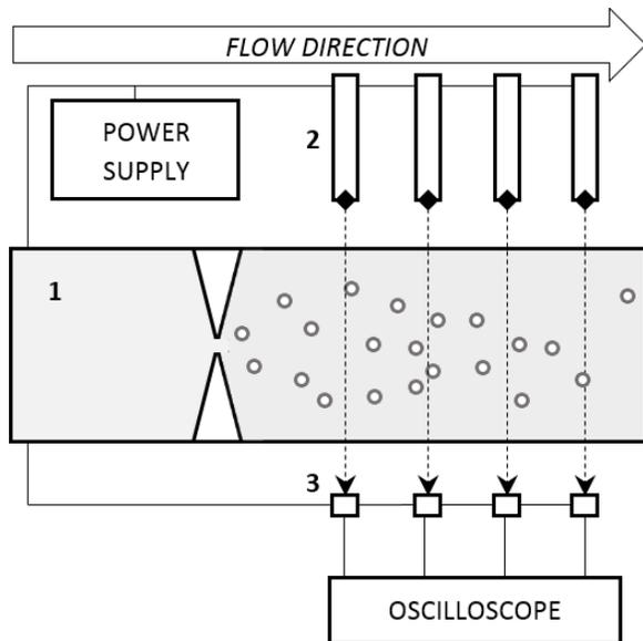
**Fig. 1.** Scheme of the measurements:
