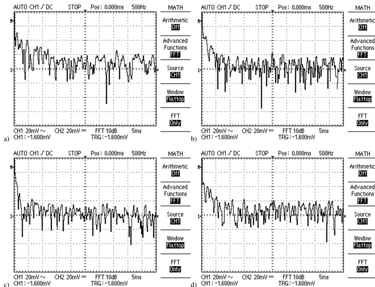
Fig. 5. The frequency spectrum obtained for the first (a), second (b), third (c) and fourth (d) photoresistor, counting from the nozzle.
