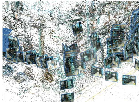
Fig. 8 Close up view of photos taken in the water treatment plant and points generated after the first alignment
