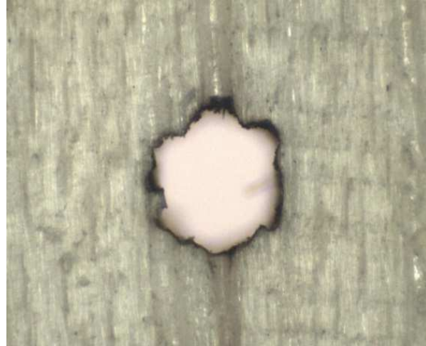
Fig. 9. Micro-perforation of sample 1M made from plywood with thickness of 3 mm using laser engraving
