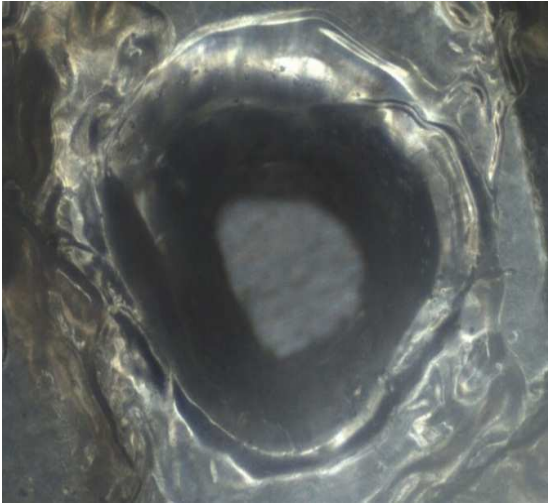
Fig. 11. Micro-perforation of sample 1M made from PC with thickness of 1 mm using laser engraver
