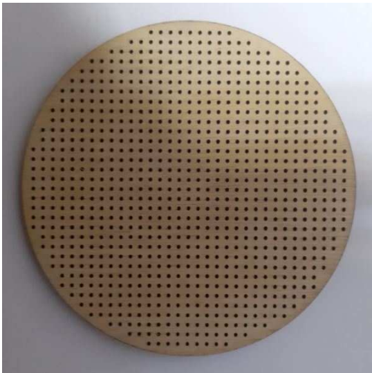
Fig. 8. Sample 1M made from plywood
