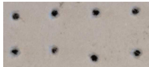
Fig. 15. Close-up of micro-perforations of cardboard sample 2M
