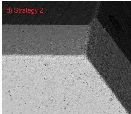
Fig. 2 a) Wet-sandblasting setup, b) Reamer sharp cutting edges, c) Microgeometry resulted after strategy 1, d) Microgeometry resulted after strategy 2
