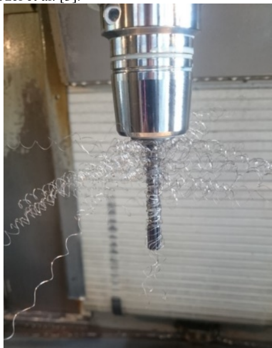
Fig. 1. Chips stringy wrapped around reamer
