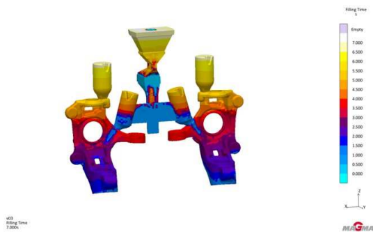
Fig. 17. Cast iron knuckle solidification analysis
