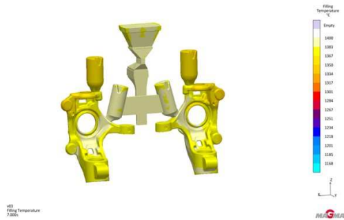
Fig. 13. Cast iron knuckle filling temperature analysis
