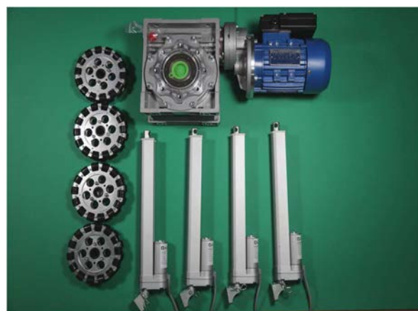
Fig. 11 The bed drive system
