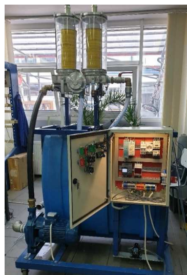
Fig. 4. Filter stand ready for testing
