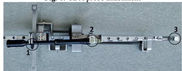
Fig. 7. RFA probe - Inappropriate Attachment
