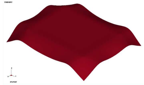
Fig. 5. Semi-finished product after gravitational deformation
