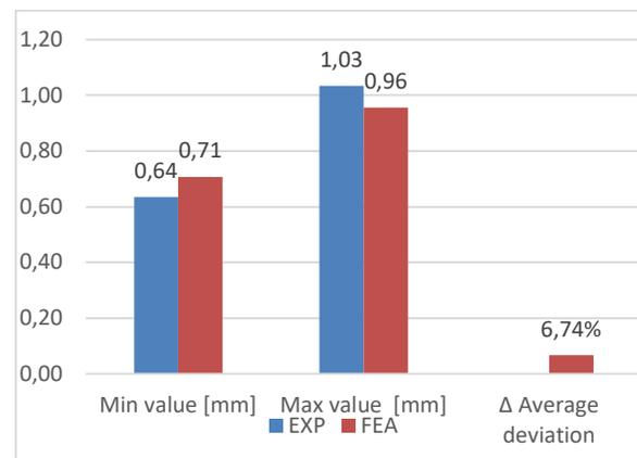
**Fig 14** Part thickness - 5 mm die radius, 15KN blank folder force
