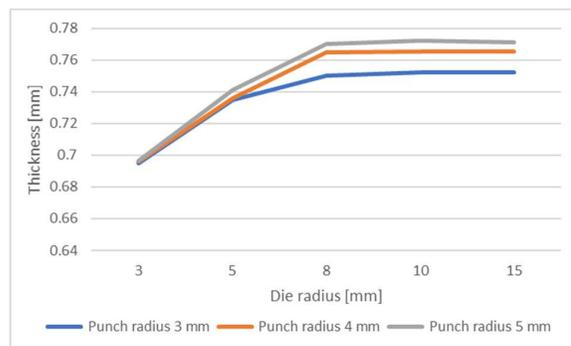
**Fig 5** Minimum thickness of the part for a blank holder force of 15 KN
