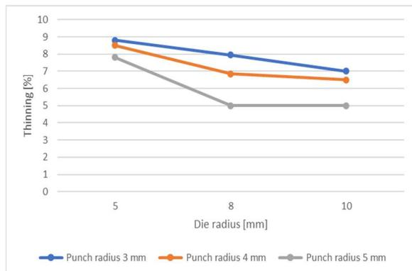
**Fig. 9** Thinning of the deep drawing part in percent for a blank holder force of 30KN
