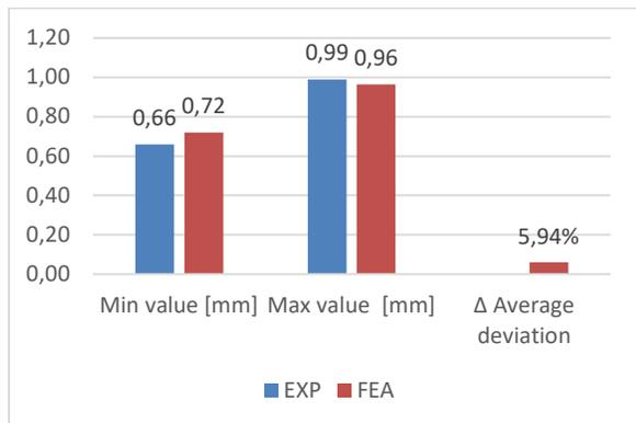
**Fig 16** Part thickness – 6.5 mm die radius, 15KN blank folder force
