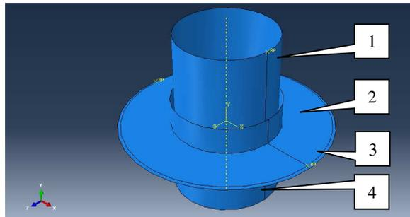
**Fig 1** 3D model of deep drawing geometry assembly 1- punch 2- blank holder 3-blank 4 -die
