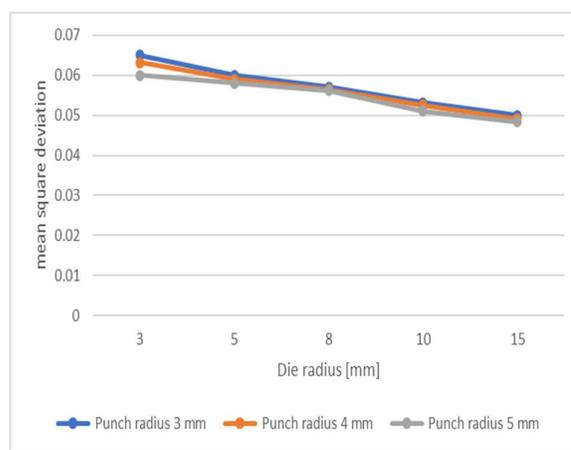
**Fig 6** The mean square deviation of the thinning of the deep drawing part for the blank holder force of 15KN
