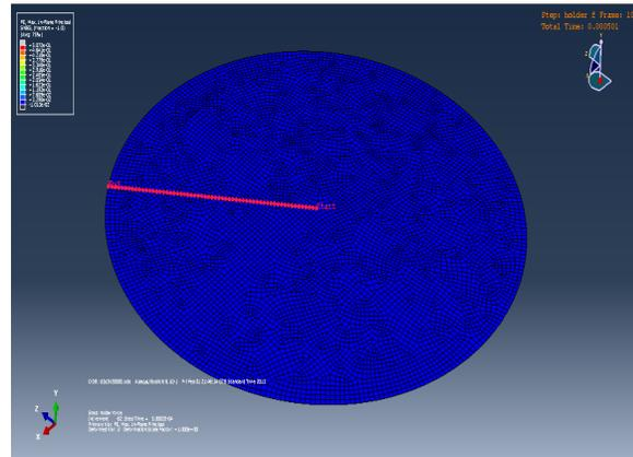
**Fig 2** The points along the radius of the blank where the measurements are made
