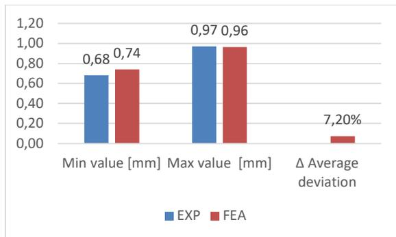
**Fig 19** Part thickness - 8 mm die radius, 30KN blank folder force
