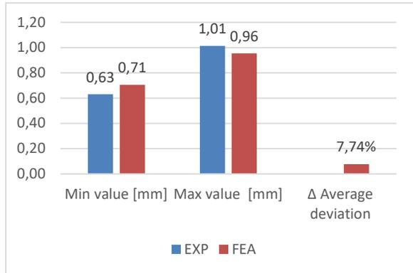
**Fig 15** Part thickness - 5 mm die radius, 30KN blank folder force
