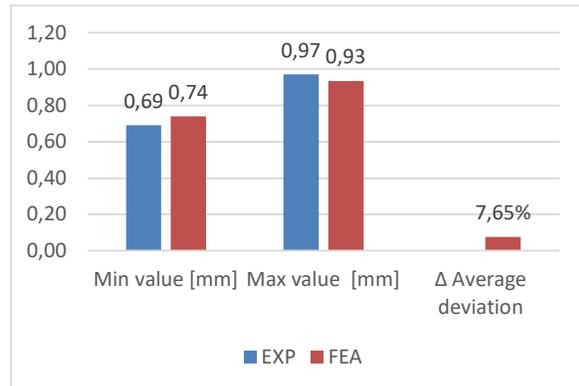
**Fig 18** Part thickness - 8 mm die radius, 15KN blank folder force
