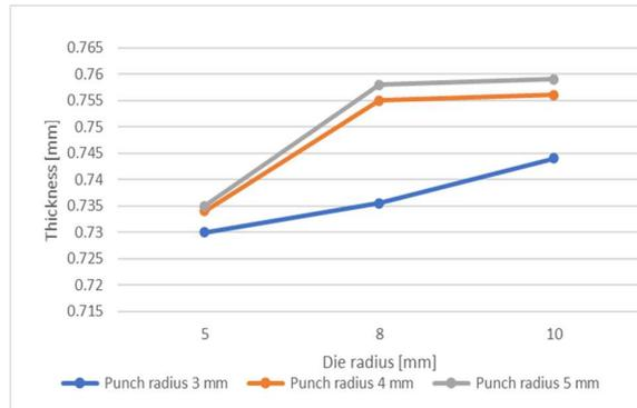
**Fig 10** Variation of the thickness of deep drawing part for different punch and die radius, blank holder force 40kN
