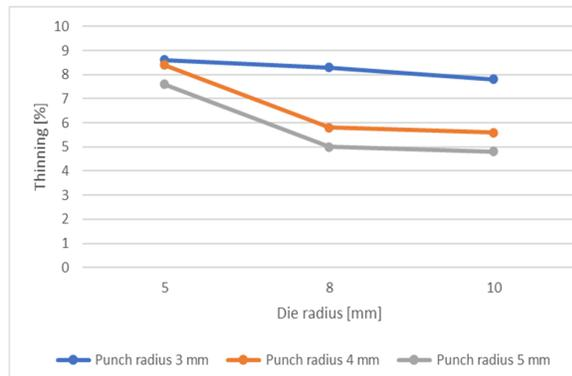
**Fig 12** Thinning of the deep drawing part in percent for a blank holder force of 40KN
