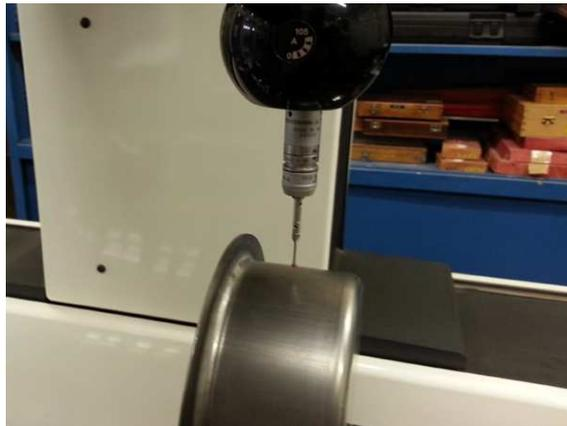
**Fig 13** Measuring the deep drawing cylindrical part with the coordinate measuring machine
