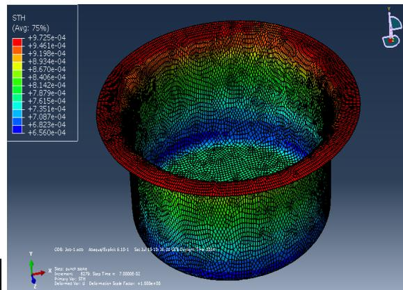
**Fig 3** Distribution of thickness variation to a deep drawing cylindrical part
