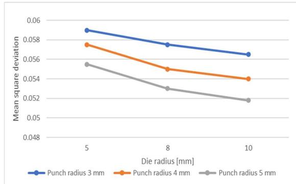
**Fig 8** The mean square deviation of the thinning of the deep drawing part for a blank holder force of 30KN
