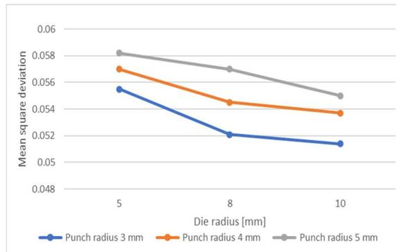
**Fig 11** The mean square deviation of the thinning of the deep drawing part for a blank holder force of 40KN
