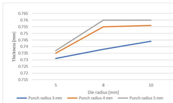
**Fig 7** Variation of the thickness of deep drawing part for different punch and die radius, blank holder force 30kN
