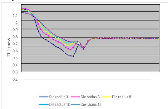
**Fig 4** Variation of the thickness of the blank for different die radius
