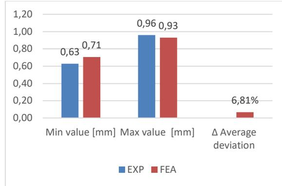
**Fig 17** Part thickness – 6.5 mm die radius, 30KN blank folder force
