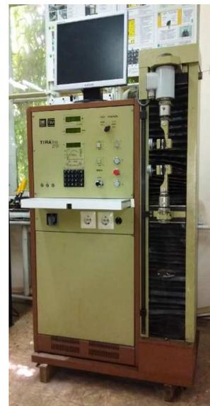
**Fig. 3.** TIRATEST 2151 Universal testing machine
