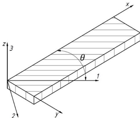
Fig. 5. Angle orientation direction and load direction
