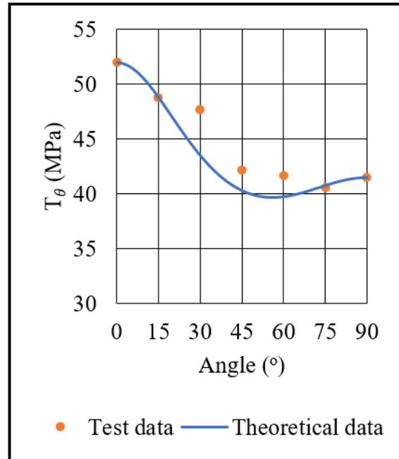
Fig. 8. UTS comparison between theoretical data and test data for materials with 0,3 mm layer thickness
