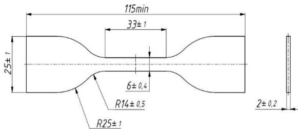
**Fig. 2.** Drawing of a Type-1 specimen
