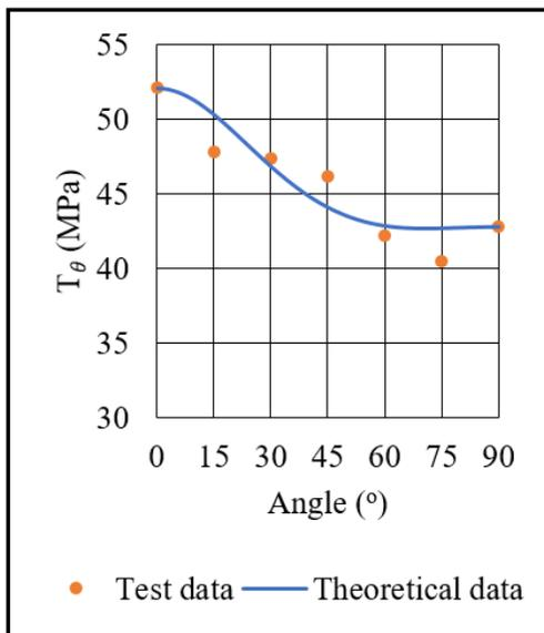
Fig. 7. UTS comparison between theoretical data and test data for materials with 0,2 mm layer thickness
