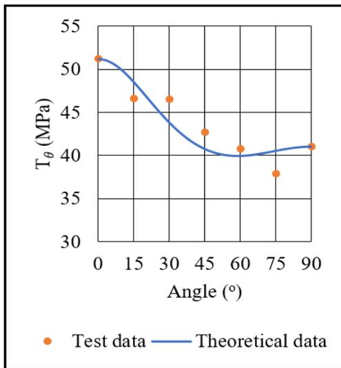
Fig. 6. UTS comparison between theoretical data and test data for materials with 0,1 mm layer thickness
