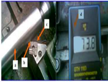
Fig. 3. Temperature measuring device. (a) workpiece , (b): plate, (c): thermocouples and (d): measuring device.
