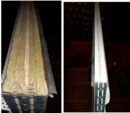
Fig. 1. Structure detail of the noise barrier model
