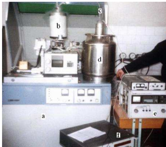
Fig.1. Experimental facility: a - DRON-3 diffractometer, b - Roentgen low temperature device URNT-180, c - nitrogen liquid transfer device, d - Dewar vessel (liquid nitrogen), e - control unit and control, f - voltmeter.
