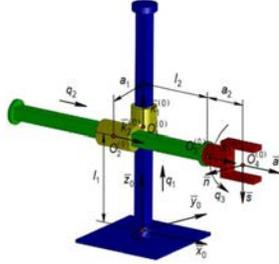
Fig. 2. The Kinematic scheme of serial robot 2TR
