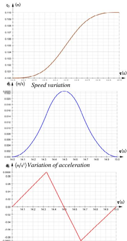
Fig. 6 Representation of kinematical parameters on sequence j=3
