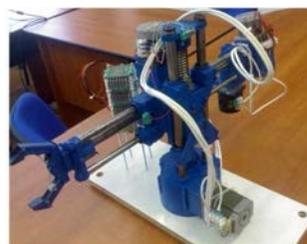
Fig. 1. The 2TR serial robot
