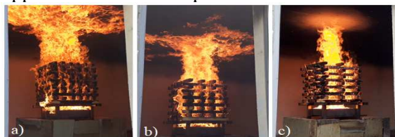
Fig. 9. Time of peak temperature in the test area in case of wood crib burning: a) model 1; b) model 2; c) model 3
