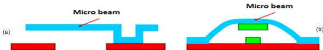
Fig. 10. Configuration of micro commutator based on a micro beam with (a) lateral contact (b) central contact.
