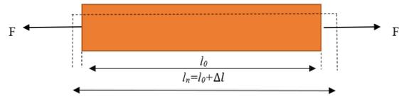
Fig. 4. Test piece subjected to tensile test:  $l_0$  length sample, tensile stress with axial forces  $F$ , the sample elongates at  $l_n$
