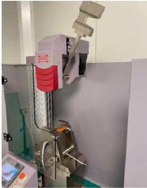
Fig. 3. Testing of ertalon 4.6 material at breaking
