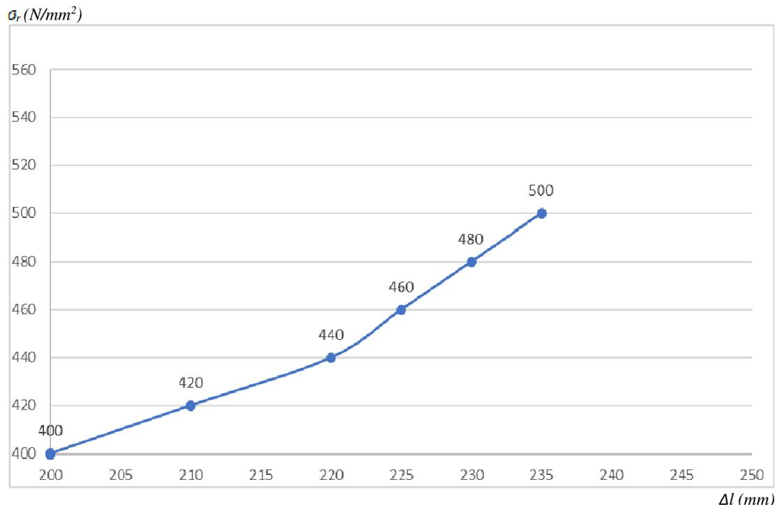
**Fig. 5.** Distribution of the tensile strengths of the ertalon 4.6 sample depending on the linear elongation at deformation
