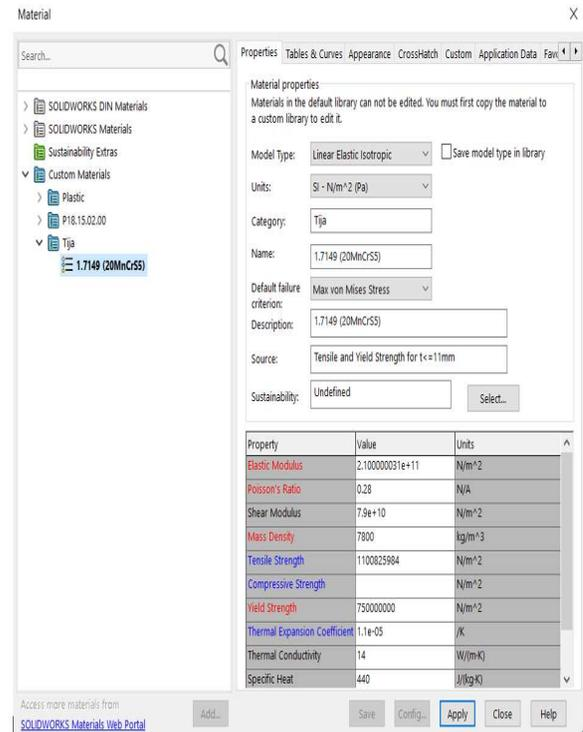
The material selection regarding the simulation is equivalent to that of the device design and are show in the table 1. FEA simulations for bending and deflection are performing in a preliminary form starting from theoretical formulas.
