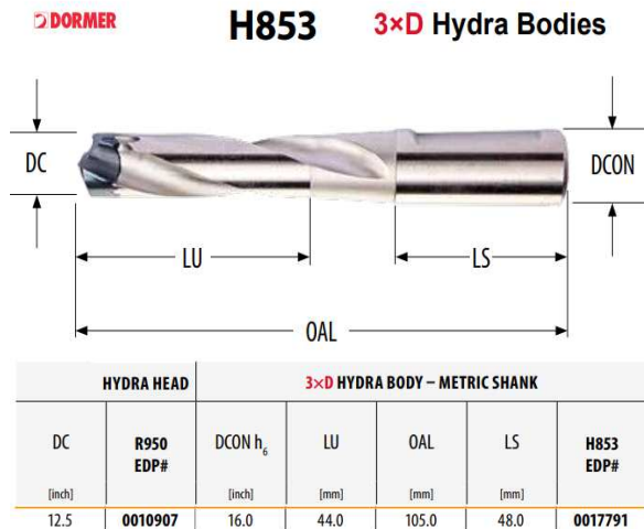
Fig. 2. The drill body dimensions [12].
