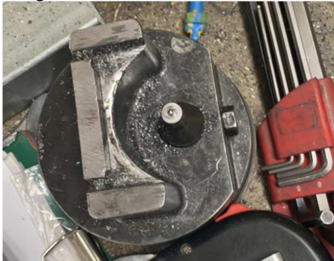
Fig. 9. The punching tool set (removed from the assembly)
