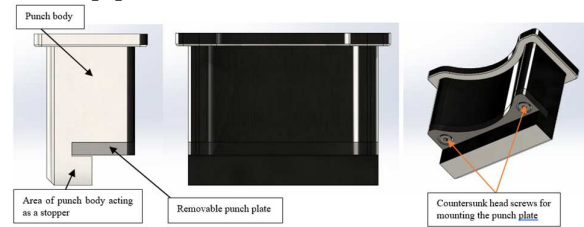
Fig. 17. The trimming punch; left view (left), front view (middle) and custom view (right)
