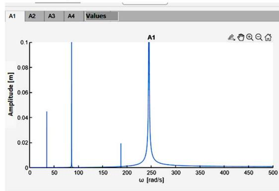
**Figure 5.** Graph for amplitude curve,  $A_1$  –PULS-AMP program
