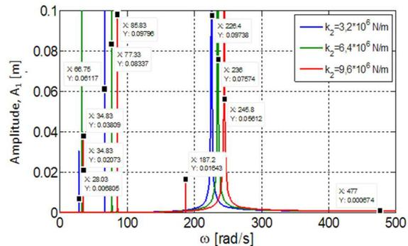
**Figure 6.** Graph for amplitude curve,  $A_1$  – MatLab program
