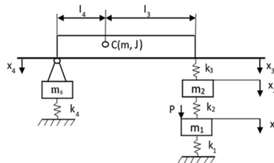
**Figure 2.** Dynamic model for the vibrating compactor
