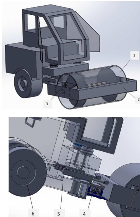
**Figure 1.** Constructive scheme for the vibrating compactor; 1 – vibratory roller; 2 – front chassis; 3 – first elastic step for vibration isolation and damping; 4 – second elastic step for vibration isolation and damping; 5 – rear chassis; 6 – propelling wheels.
