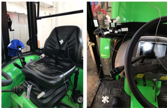
Fig. 3. Mounting of tri-axial accelerometers on the surface of the tractor seat, on the seat back and the base of the cab near the driver's support leg.
