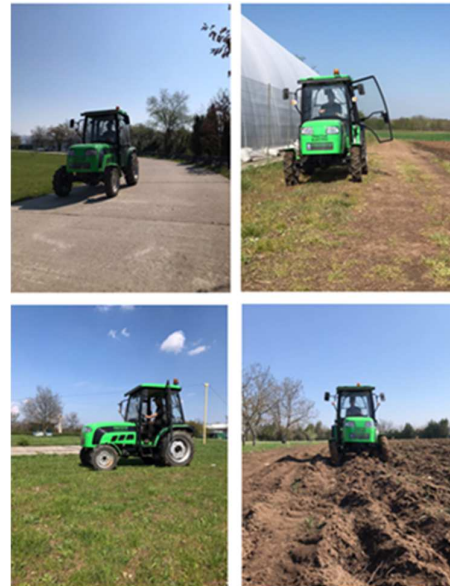
Fig. 2. Description of the protocol regarding the experimental tests performed on the 4 types of road at constant speed of 5 km/h: a) straight terrain; b) uneven ground; c) uncultivated land; d) plowed land
