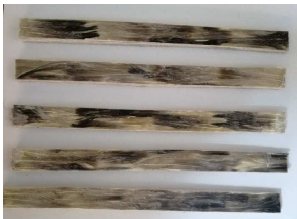
Fig. 5. The samples from chicken feathers/sheet of cellulose fibers and Crystal super transparent resin for tensile test
