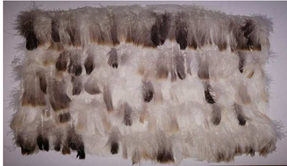
Fig. 1. Crystal super transparent resin and chicken feathers/sheet of cellulose fibers layer
