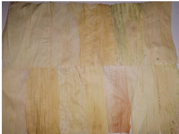
Fig. 3. Crystal super transparent resin and corn ear leaves/sheet of cellulose fibers layer
