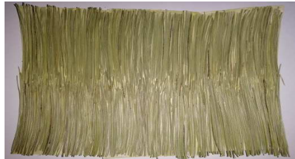
Fig. 4. The final material made with Crystal super transparent resin and needles from tree firs/sheet of cellulose fibers layer
