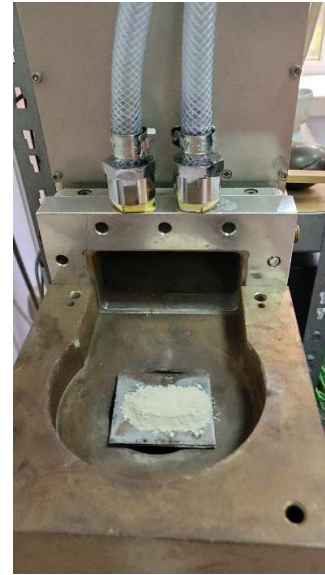
Fig. 5 Powder into the microwave furnace before preheating process
