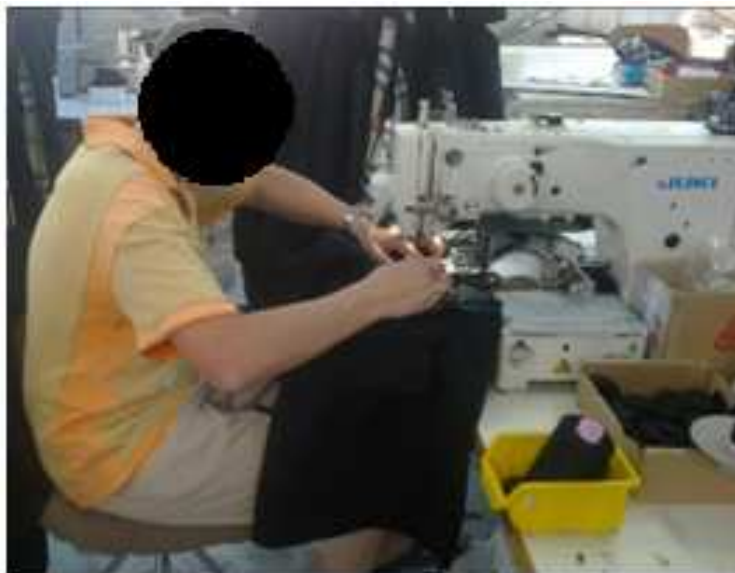
Fig. 4. Sewing the leather logo (semi-automatic sewing machine).
