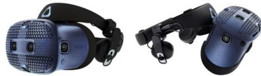
Fig. 3. HTC Cosmos VR Headset with built in flipping visor and adjustable headphones [11]
