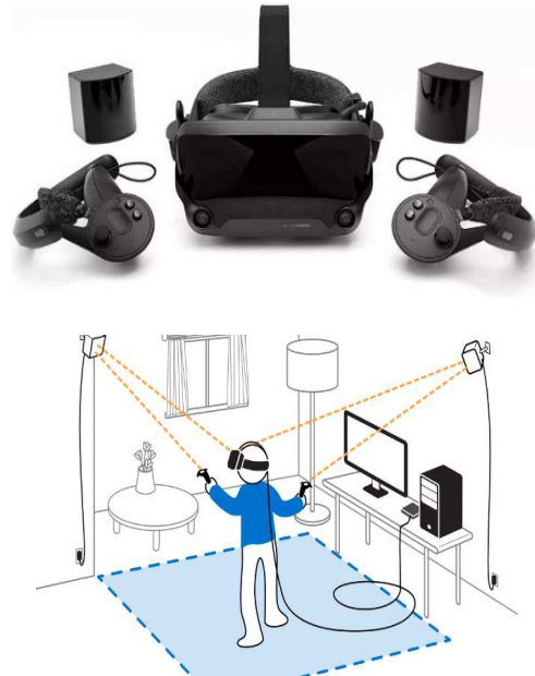
Fig. 4. Valve Index VR Headset presented at the top and the ideal room setup using two base station sensors presented at the bottom [11]
