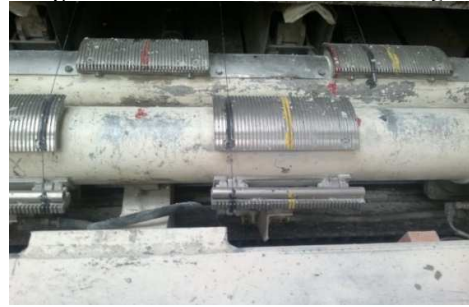
Fig. 6. Detail cross-cutting wires on oscillators.
