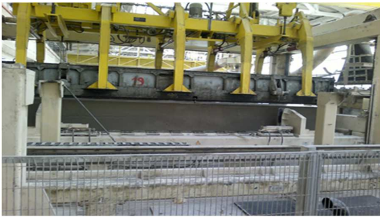
Fig.1. Laying the concrete block on the cutting machine.
