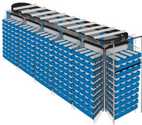
Fig. 1. Stand-alone horizontal carousel unit [22].
