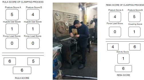
Fig. 7. Risk scores of clamping processes while the operator turns the product by force.
