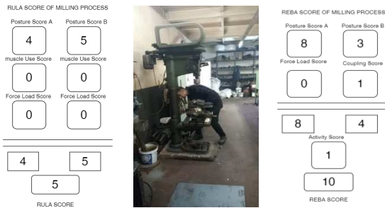
Fig. 9. Risk scores of milling processes while the operator is bending over.
