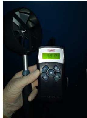
Fig. 2. KIMO LV 110 anemometer during measurements.
