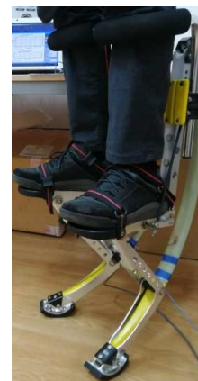
Fig. 3. Highlighting the variable cross-section of the elastic element.
