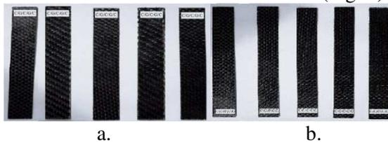
**Fig. 2.** Sets of five composite hybrid laminated test specimens: a. [CF/GF/CF/GF/CF]; b. [CF/CF/GF/CF/CF].
