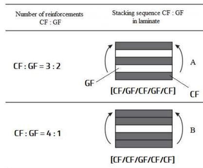
**Fig. 1.** Stacking sequences for carbon and glass sheets.
