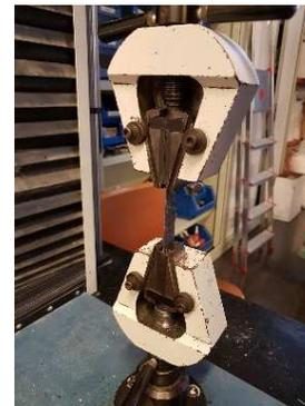
**Fig. 4.** Fixing mode of the test piece on the universal electromechanical testing machine type ELIB 50.
