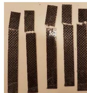
**Fig. 5.** Sample set of specimens [CF / GF / CF / GF / CF] broken after tensile stress.
