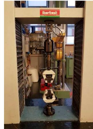
**Fig. 3.** Universal electromechanical testing machine type ELIB 50.
