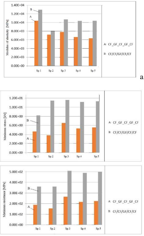
**Fig.7.** Values of experimentally analyzed parameters: a. modulus of elasticity; b. maximum stress; c. maximum resistance.
