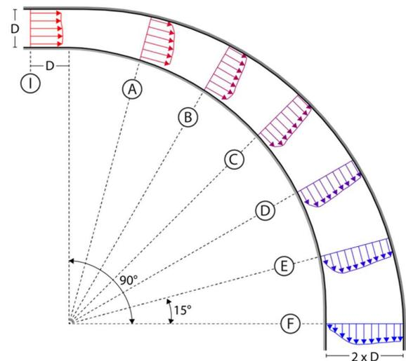
**Fig. 6.** Curved diffuser geometry and flow profiles based on real velocity data presented by Majumdar et al. [17]
