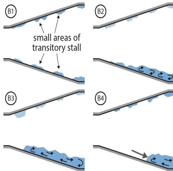
**Fig. 4.** Diffuser in various stages in the stall-wash-out cycle within transitory stall. Adapted from [13].
