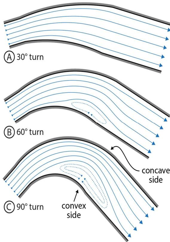
**Fig. 5.** Stall regime in curved diffusers. With an increasing expansion angle, the flow separation moves upstream and increases in magnitude. Adapted from [15].
