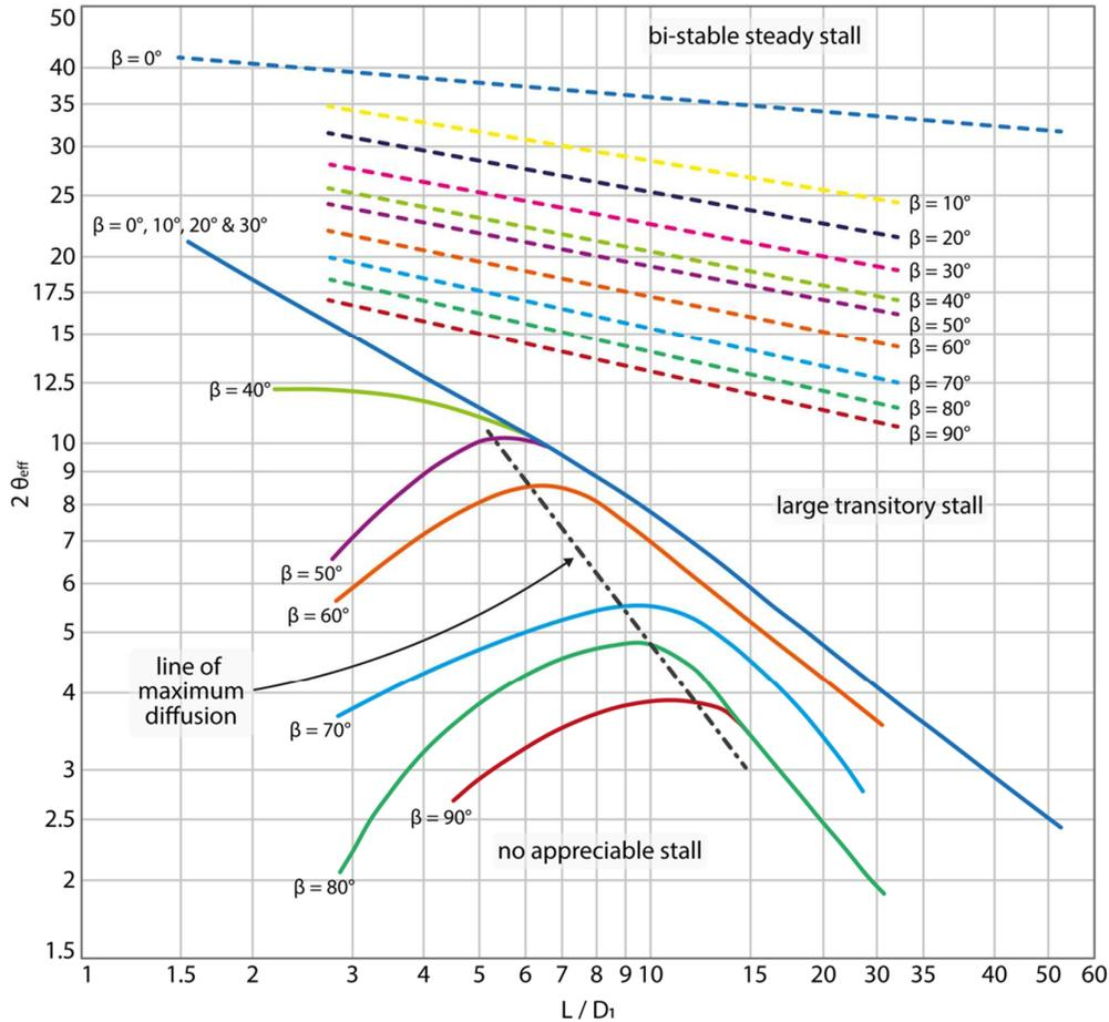
**Fig. 7.** Stall behaviour mapped over normalised diffuser size ( $L/D_1$ ) and total effective expansion angle ( $2\theta_{eff}$ ) for curved diffusers with varying turning angles  $\beta$ . Solid lines mark the lower boundary of the transitory stall regions, while dotted lines represent the upper boundary. Also included, is the line along which the lowest  $L/D_1$  results in the maximum level of diffusion. Adapted from [14].
