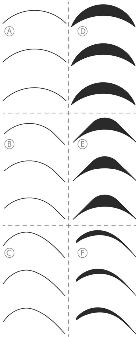
**Fig. 1.** Flat-plate (left) and profiled (right) vanes. These will be referred to as  $\frac{1}{4}$  circle vanes (A),  $\frac{1}{4}$  circle vanes with an extended trailing edge (B), Kröber vanes (C), crescent vanes (D), constant channel vanes (E) and KTH (Royal Institute of Stockholm) vanes (F). All vanes shown share a common chord length.
