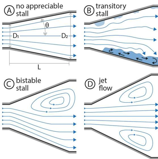
**Fig. 3.** Diffusers with increasing (from A to D) angle  $\theta$  and resulting flow regimes. Adapted from [11, 12].
