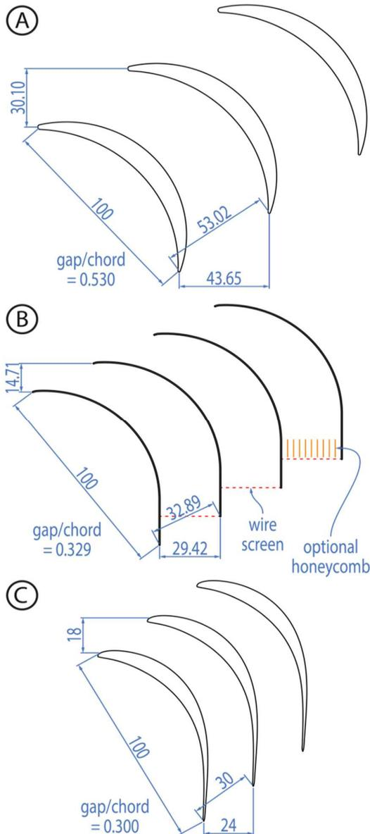
**Fig. 8.** Comparison of pitch, shape and setup of expansion vanes by Friedman et al. (A), Drela et al., (B) and Lindgren et al. (C). All vanes are scaled to have the same chord length for comparative purposes.
