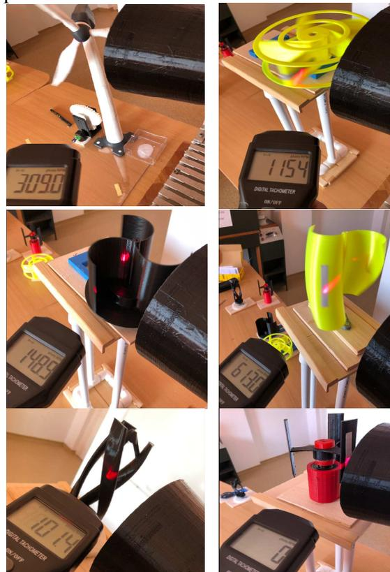
**Fig. 12.** Measurement for different geometries of wind turbines
