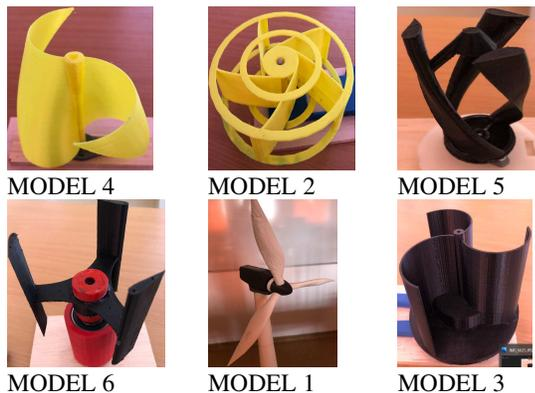
Fig. 6. Different types of wind turbines with horizontal and vertical axis, made on 3D printers
