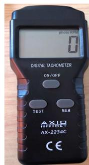
**Fig. 8.** Digital tachometer, model AX 2234C used to determine the number of rotations of printed wind turbines
