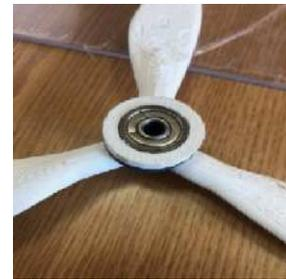
**Fig. 9.** Example of fastening bearings to the axis of printed wind turbines
